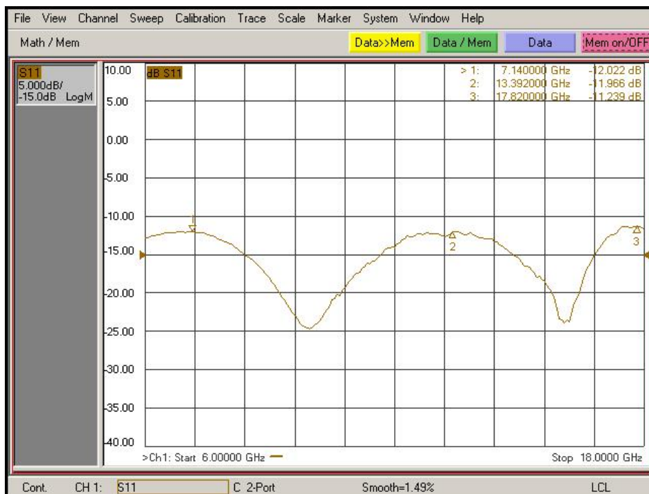
Input Return Loss, S11 Curve Test, Pin=-30dBm && Pin=0dBm [Load VSWR ≤ 1.2]
