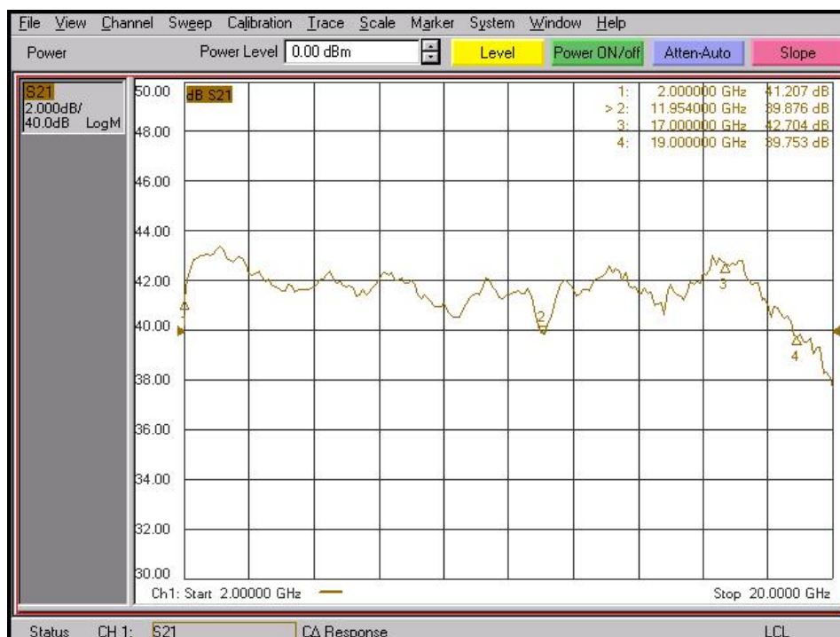
Graph2: Power Gain @ Pin=0 dBm (Ambient temp. +25±3°C, LOAD VSWR ≤ 1.3)
