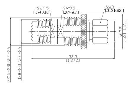
All dimensions are in mm [inch] Tolerances according to DIN ISO 2768-mH
