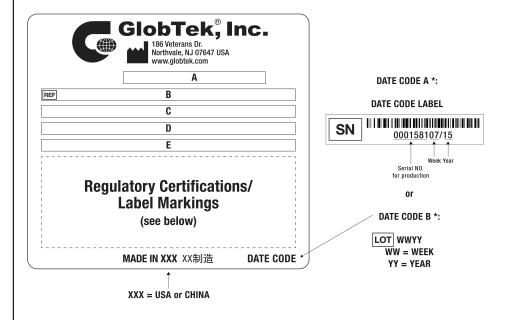
A=ICT / ITE / Medical Power Supply B=P/N: (料号) GTM91128LI1C1000T00 C=Model (型号) GTM91128LI1CEL D=Input (输入)100-240V~, 50-60 Hz, 1.5A E=Output (输出)4.2 V == 1.0 A, 4.20W
