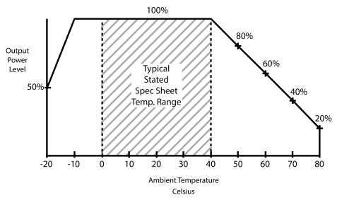
Drawing Title: GTM91128LI1CEL, ICT / ITE / Medical Power Supply, Efficiency Level: N/A, Case Color/Style: GlobTek Black, Wall Plug-in+Desktop Combination, Li-Ion Battery Charger, Input Rating: 100-240V~, 50-60 Hz, IEC 60320/C8, , Output Rating: 4.20W, 4.2V@1.0A, Pin Out: Polarity Configuration T00 All plugs are Medical Grade, Locking, Polarized once installed, and single use only. Product demonstration link:
