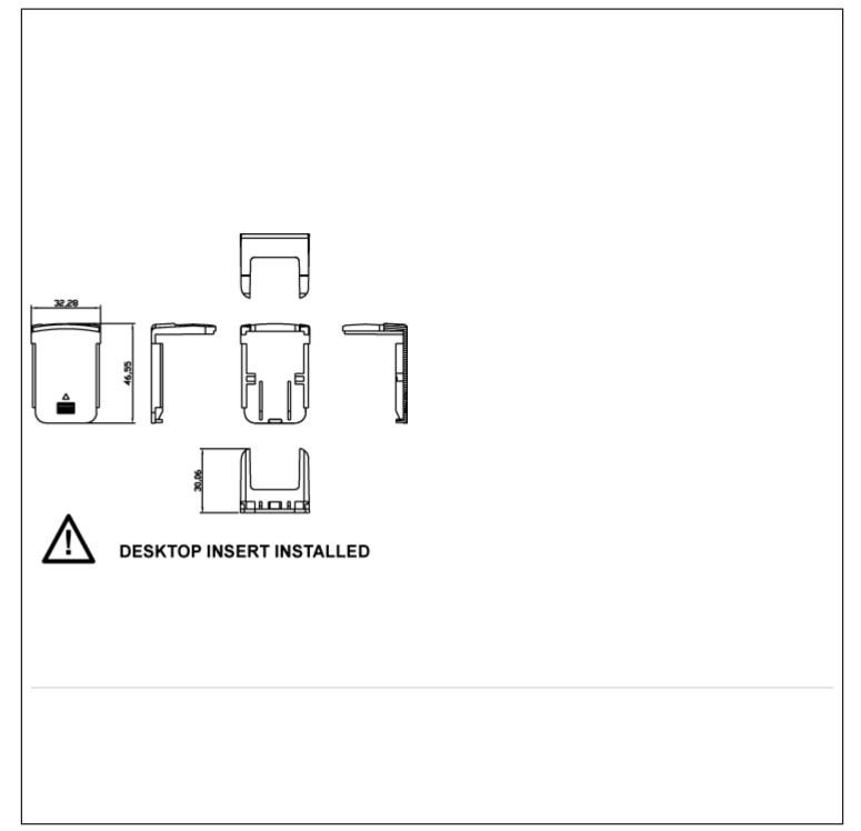
Drawing Title: GTM91128LI1CEL, ICT / ITE / Medical Power Supply, Efficiency Level: N/A, Case Color/Style: GlobTek Black, Wall Plug-in+Desktop Combination, Li-Ion Battery Charger, Input Rating: 100-240V~, 50-60 Hz, IEC 60320/C8, , Output Rating: 4.20W, 4.2V@1.0A, Pin Out: Polarity Configuration T00 All plugs are Medical Grade, Locking, Polarized once installed, and single use only. Product demonstration link:
