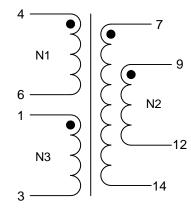
N2 denotes 2 windings connected in parallel. Terminals 7+9 and 12+14 must be tied as solder bridging is allowed.
