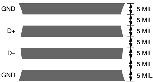
Figure 21. Typical Arrangement of Signal Tracks
