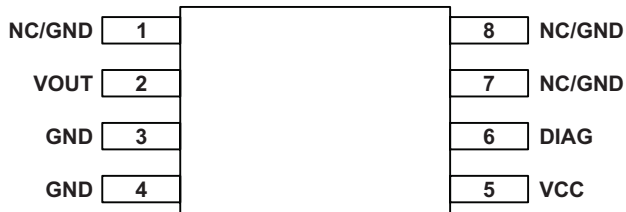
Package LE, 8-Pin eTSSOP Pinouts
