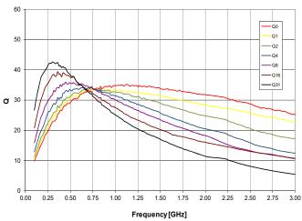
Figure 12. Measured Shunt Q (state 31) vs. Frequency (temperature)
