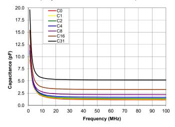
Figure 13. Measured Shunt C vs. Frequency (major states, 1 MHz - 100 MHz)
