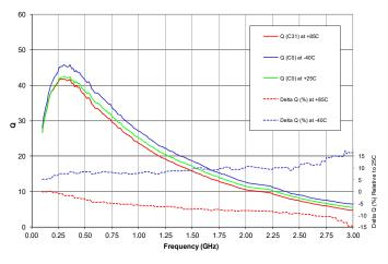
Figure 11. Measured Shunt Q (state 0) vs. Frequency (temperature)
