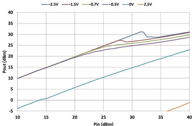
Figure 9.  $P_{OUT}$  vs.  $P_{IN}$  Over Frequency @  $V_{CTRL} = -0.7V$
