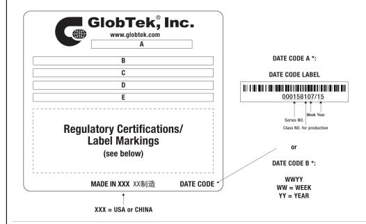
A=PoE, Passive Power Injector B=P/N: (料号) GT-96180-1818-T3-PP C=Model (型号) GT-96180-1830-12.0-T3-PP D=Input (输入)100-240V~, 50-60 Hz, 0.6A E=Output (输出)18.0 V == 1.0 A, 18.00W
