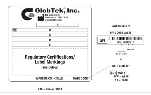
A=ICT / ITE / Medical Power Supply B=P/N: (料号) TR9CI5000YL4CIMR6B C=Model (型号) GTM961200P12024-T3 D=Input (输入)100-240V~, 50-60 Hz, 1.5 A E=Output (输出)24.0 V === 5.0 A, 120.00W
