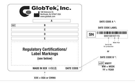
A=ICT / ITE / Medical Power Supply B=P/N: (料号) TR9CX2500T00-IM(R6B) C=Model (型号) GTM961200P12048-T3 D=Input (输入)100-240V~, 50-60 Hz, 1.5 A E=Output (输出)48.0 V == 2.5 A, 120.00W
