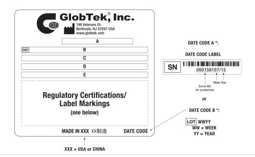
A=Medical/ICT/ITE/Household use Power Supply B=P/N: (料号) RR9LH2000T00NACIMR6B C=Model (型号) GTM96300-3619.5-1.5-R3A D=Input (输入)100-240V~, 50-60 Hz, 1.0A E=Output (输出)18.0 V === 2.0 A, 36.00W
