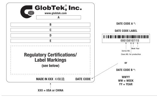
A=ICT/ITE Power Supply B=P/N: (料号) TR9KG1600CCP-N(R6B) C=Model (型号) GT-46240-2415-T2 D=Input (输入)100-240V~, 50-60 Hz, 0.6 A E=Output (输出)15.0 V == 1.6 A, 24.00W
