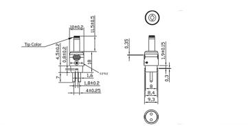
Option upon request: STRAIGHT Female Barrels are available for special order in any length between 9mm-14mm
