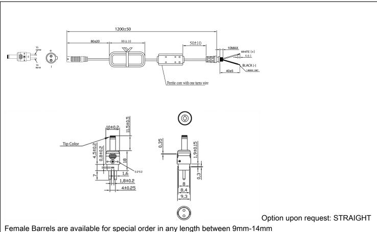
This novel system allows for rapid shipment of prototype samples or small quantities of common output voltage and current which can fulfill the needs of most common barrel plug as well as male plug specs. The table explains the standard and non-standard options available as part of this system. This system also allows for both Center Positive and Center Negative
