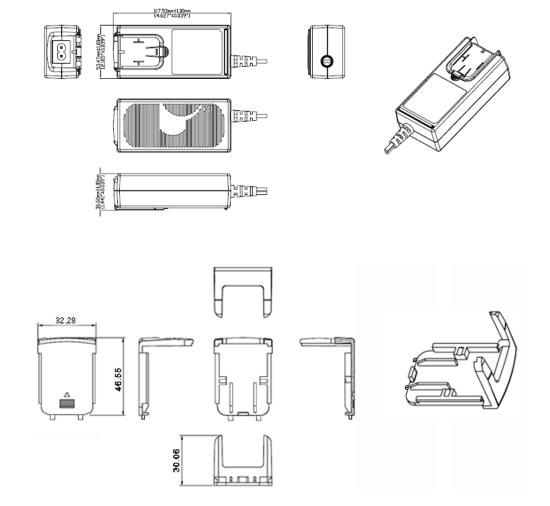
Unit shipped without an installed input plug.
