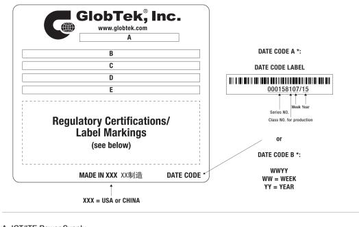
A=ICT/ITE Power Supply B=P/N: (料号) TR9CG1600LCP-N(R6B) C=Model (型号) GT-46240-2415-T3 D=Input (输入)100-240V~, 50-60 Hz, 0.6 A E=Output (输出)15.0 V === 1.6 A, 24.00W
