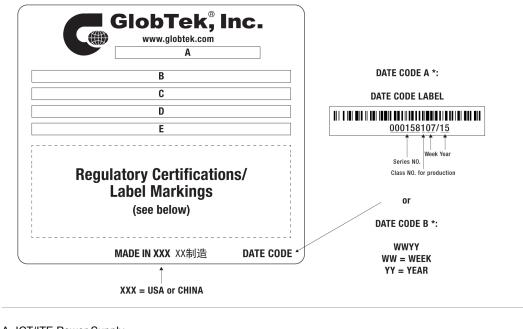
A=ICT/ITE Power Supply B=P/N: (料号) TR9CG1600CCP-N(R6B) C=Model (型号) GT-46240-2415-T3 D=Input (输入)100-240V~, 50-60 Hz, 0.6 A E=Output (输出)15.0 V === 1.6 A, 24.00W
