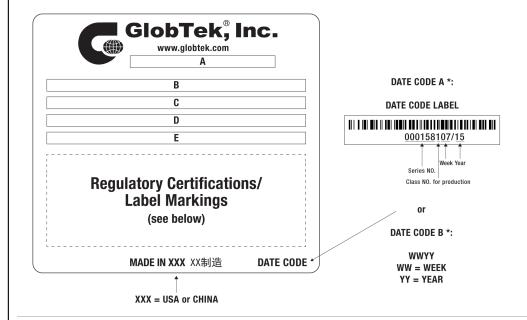
A=ICT / ITE / Medical Power Supply/Class 2/Household Power Supply B=P/N: (料号) WR9QI250T00NAIMR6B C=Model (型号) GTM96060-0624 D=Input (输入)100-240V~, 50-60 Hz, 0.6 A E=Output (输出)24.0 V === 0.25 A, 6.00W
