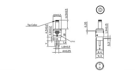
Option upon request: STRAIGHT Female Barrels are available for special order in any length between 9mm-14mm
