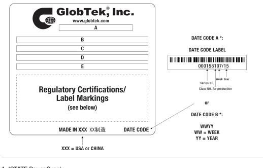
A=ICT/ITE Power Supply B=P/N: (料号) WR9QE3000LCP-N(R6B) C=Model (型号) GT-46401-3612 D=Input (输入)100-240V~, 50-60 Hz, 1.0A E=Output (输出)12.0 V === 3.0 A, 36.00W
