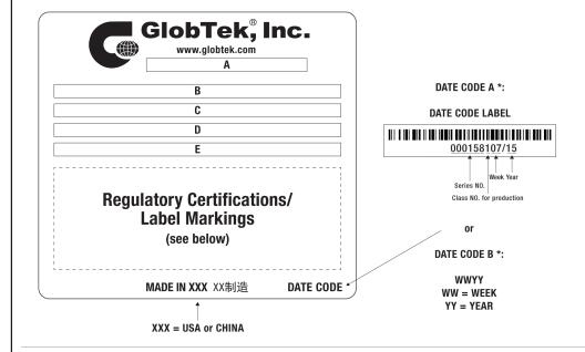
A=ICT / ITE / Medical Power Supply/Class 2/Household Power Supply B=P/N: (料号) TR9CA3600LCP-IMR6B C=Model (型号) GTM96180-1807-2.0-T3 D=Input (输入)100-240V~, 50-60 Hz, 0.6 A E=Output (输出)5.0 V ---- 3.6 A, 18.00W
