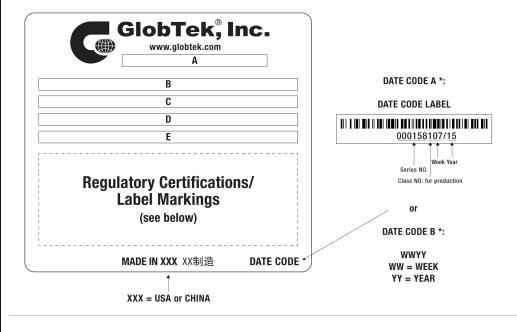
A=ICT/ITE Power Supply B=P/N: (料号) WR9HE2000L9P-F(R6B) C=Model (型号) GT-86240-2412-W2 D=Input (输入)100-240V~, 50-60Hz, 0.8A E=Output (输出)12.0 V == 2.0 A, 24.00W
