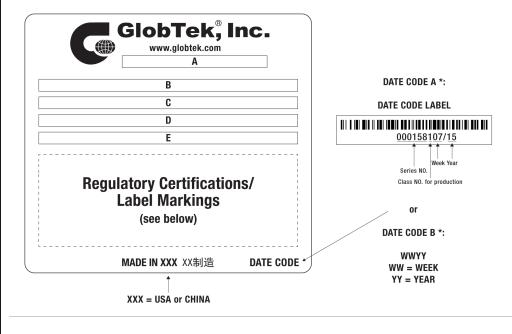
A=ICT/ITE Power Supply B=P/N: (料号) TR9CA3000CCP-N(R6B) C=Model (型号) GT-46181-1505-T3 D=Input (输入)100-240V~, 50-60 Hz, 0.5A E=Output (输出)5.0 V == 3.0 A, 15.00W
