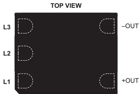
**TPM1714 VIA – PCB Mount – Pins Down**
