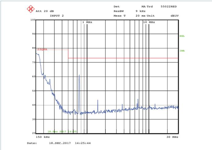
Figure 1 — Typical conducted emissions, peak scan, with BCM4414VGOF4440T02 VIA, 400V<sub>AC</sub> 90% load, no external components
