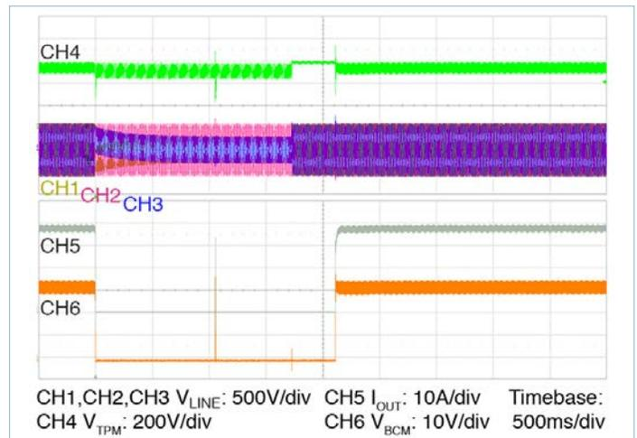
Figure 6 — Input line drop and recovery
