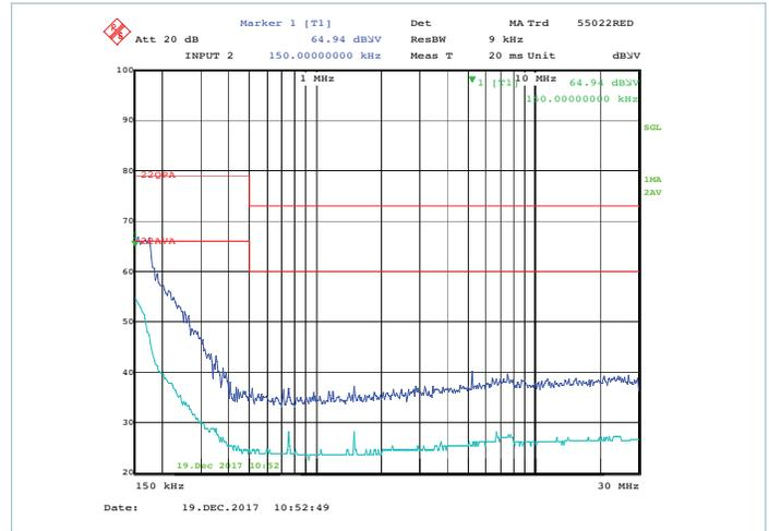
Figure 2 — Typical conducted emissions, peak and average scan, with BCM4414VGOF4440T02 VIA, 400V<sub>AC</sub> 90% load, with external components as shown in typical application on page 3
