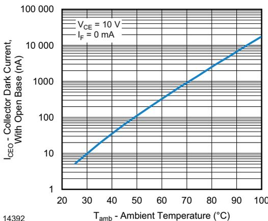
Fig. 7 - Collector Dark Current vs. Ambient Temperature
