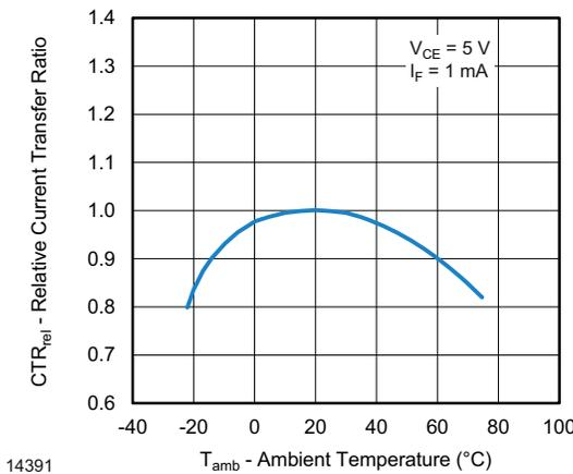
Fig. 6 - Relative Current Transfer Ratio vs. Ambient Temperature
