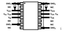
Figure 19. Recommended PCB Layout for ADuM220N/ADuM221N
