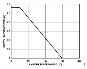
Figure 5. ADuM220N/ADuM221N Thermal Derating Curve, Dependence of Safety Limiting Values with Ambient Temperature per DIN EN IEC 60747-17 (VDE 0884-17)
