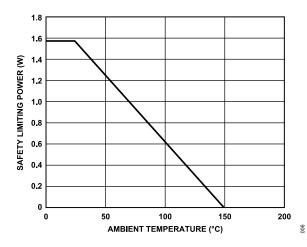
Figure 6. ADuM225N/ADuM226N Thermal Derating Curve, Dependence of Safety Limiting Values with Ambient Temperature per DIN EN IEC 60747-17 (VDE 0884-17)
