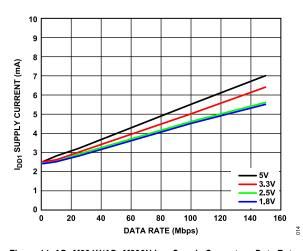
Figure 14. ADuM221N/ADuM226N I<sub>DD1</sub> Supply Current vs. Data Rate at Various Voltages
