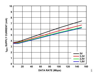
Figure 11. ADuM220N/ADuM225N I<sub>DD1</sub> Supply Current vs. Data Rate at Various Voltages
