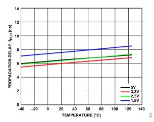
Figure 13. Propagation Delay for Logic High Output (t<sub>PLH</sub>) vs. Temperature at Various Voltages
