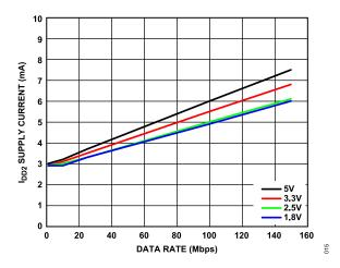
Figure 15. ADuM221N/ADuM226N  $I_{\rm DD2}$  Supply Current vs. Data Rate at Various Voltages
