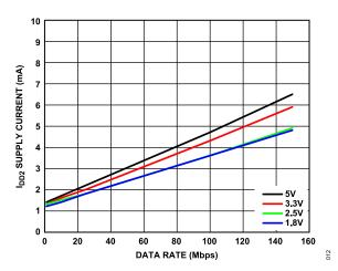
Figure 12. ADuM220N/ADuM225N  $I_{\rm DD2}$  Supply Current vs. Data Rate at Various Voltages
