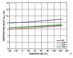
Figure 16. Propagation Delay for Logic Low Output (t<sub>PHL</sub>) vs. Temperature at Various Voltages
