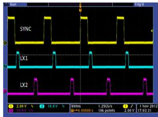
Figure 31. Synchronization at 500 kHz
