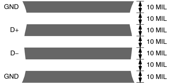
Figure 18. Arrangement of Signal Tracks
