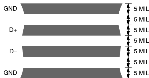
Figure 28. Arrangement of Signal Tracks
