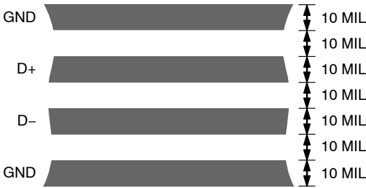
Figure 19. Arrangement of Signal Tracks
