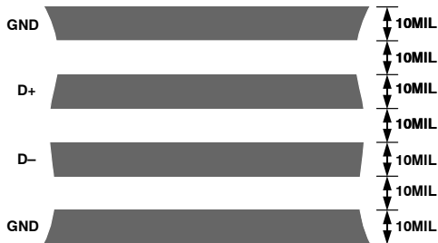
Figure 19. Arrangement of Signal Tracks
