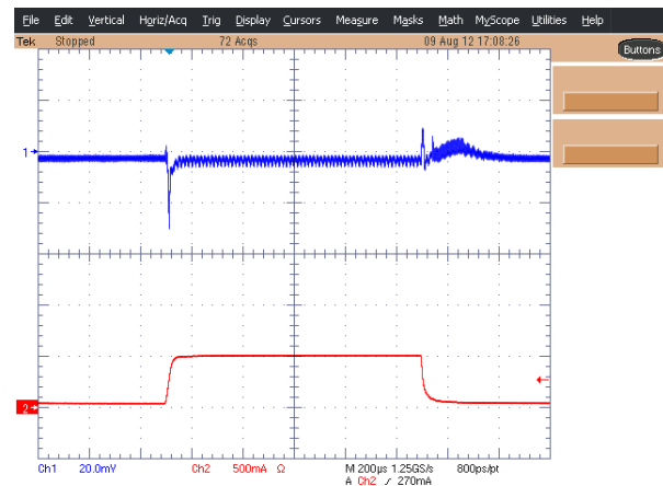
Figure 74. DCDCx Load Transient Response, 1.5 V_{OUT} , 50-500 mA Load
