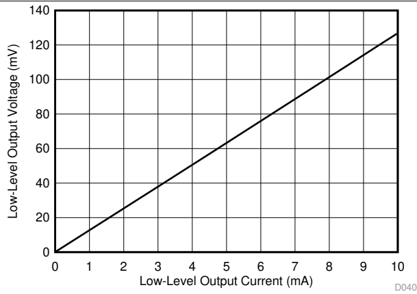
Figure 37. Low-Level Output Voltage vs Low-Level Output Current
