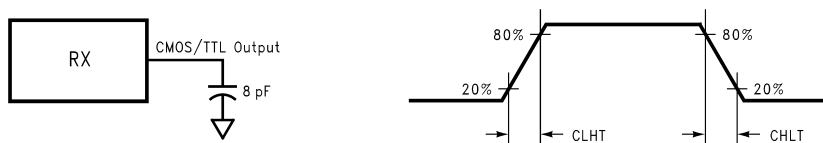
Figure 7. LVC MOS/LVTTL Output Load and Transition Times
