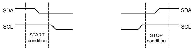
Figure 14-3. START and STOP Conditions
