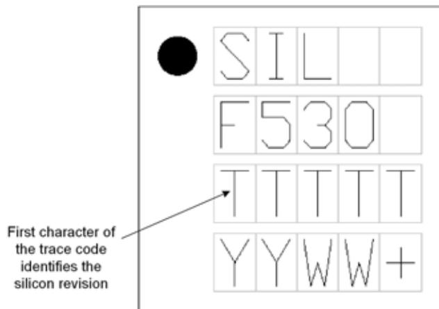
Figure 20.2. Device Package—QFN 20
