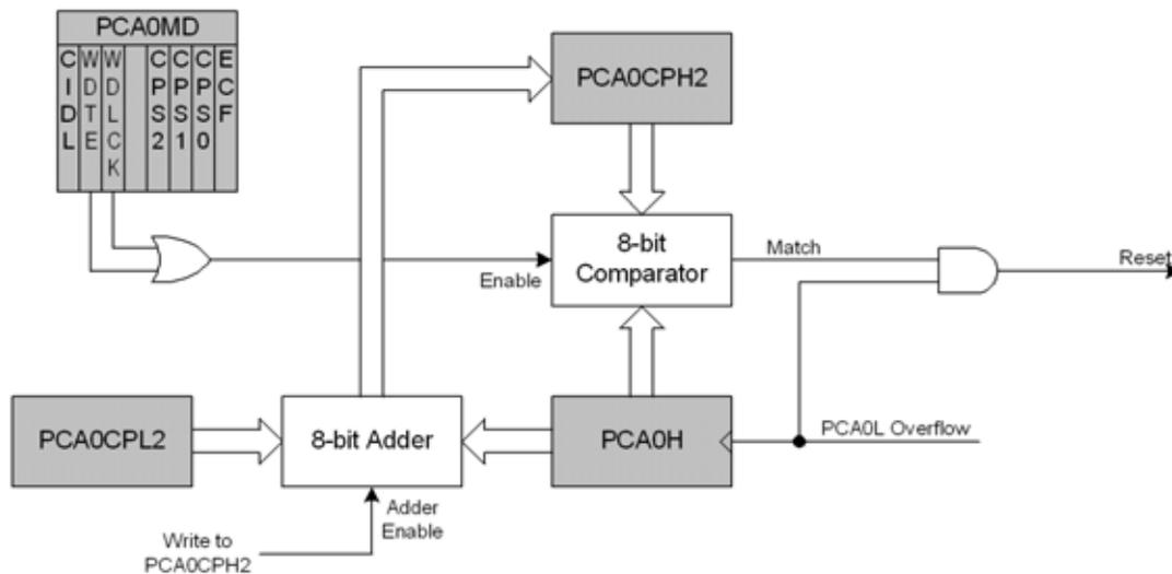
**Figure 19.10. PCA Module 2 with Watchdog Timer Enabled**
