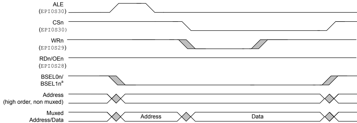
Figure 11-14. Host-Bus Write Cycle with Multiplexed Address and Data, MODE = 0x0, WRHIGH = 0, RDHIGH = 0
