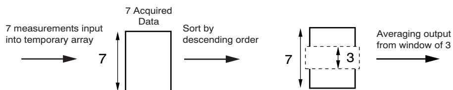
Figure 28. MAV Filter Operation (Patent Pending)
