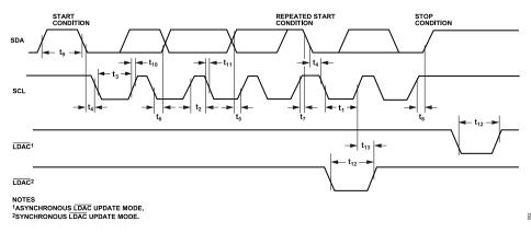
Figure 2. 2-Wire Serial Interface Timing Diagram
