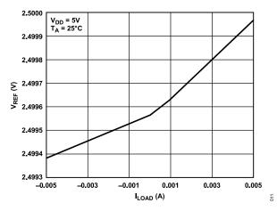
Figure 9. Internal Reference Voltage vs. Load Current
