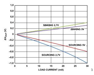
Figure 25. Headroom/Footroom vs. Load Current
