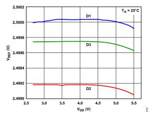
Figure 10. Internal Reference Voltage vs. Supply Voltage
