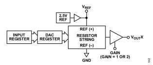
Figure 40. Single DAC Channel Architecture Block Diagram
