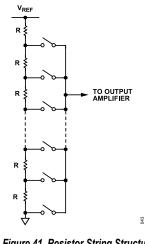
Figure 41. Resistor String Structure
