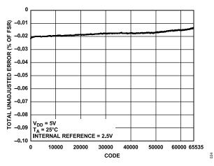
Figure 22. Total Unadjusted Error vs. Code
