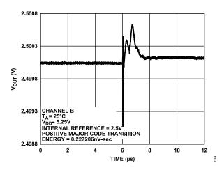
Figure 32. Digital-to-Analog Glitch Impulse
