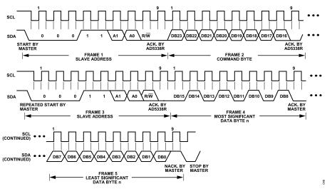
Figure 44. I<sup>2</sup>C Read Operation
