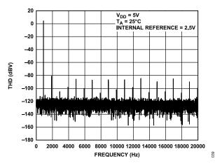
Figure 37. Total Harmonic Distortion at 1 kHz
