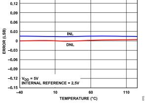
Figure 13. INL Error and DNL Error vs. Temperature
