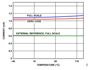
Figure 28. Supply Current vs. Temperature
