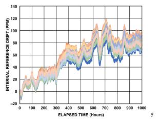
Figure 48. Reference Drift Through to 1000 Hours
