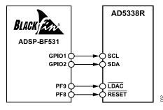
Figure 50. ADSP-BF531 Interface to the AD5338R
