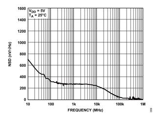
Figure 7. Internal Reference Noise Spectral Density vs. Frequency
