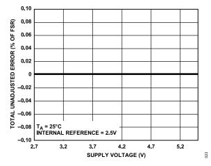
Figure 21. Total Unadjusted Error vs. Supply Voltage, Gain = 1
