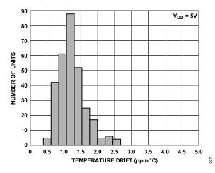
Figure 6. Reference Output Temperature Drift Histogram
