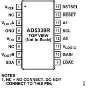
Figure 4. 16-Lead TSSOP Pin Configuration
