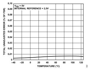
Figure 20. Total Unadjusted Error vs. Temperature
