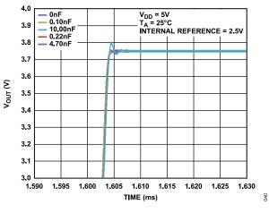
Figure 38. Settling Time vs. Capacitive Load
