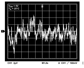
Figure 8. Internal Reference Noise, 0.1 Hz to 10 Hz
