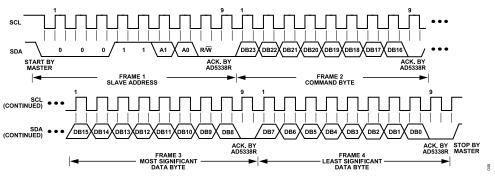
Figure 43. I<sup>2</sup>C Write Operation
