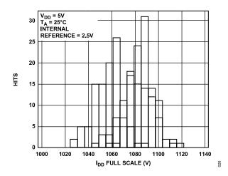
Figure 24. I<sub>DD</sub> Histogram with Internal Reference, V<sub>REFOUT</sub> = 2.5 V, Gain = 2
