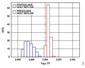
Figure 47. SHR Reference Voltage Shift
