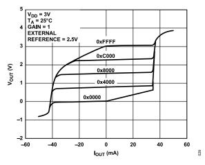
Figure 27. Source and Sink Capability at V<sub>DD</sub> = 3 V
