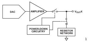
Figure 45. Output Stage During Power-Down
