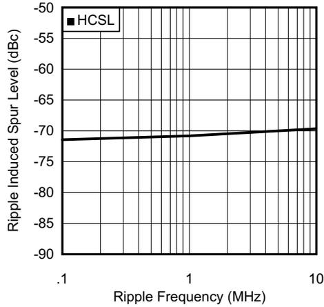
$F_{clk} = 156.25\text{ MHz}$   $V_{cc0}\text{ Ripple} = 100\text{ mV}_{pp}$
