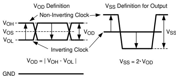
Figure 7-2. Two Different Definitions for Differential Output Signals
