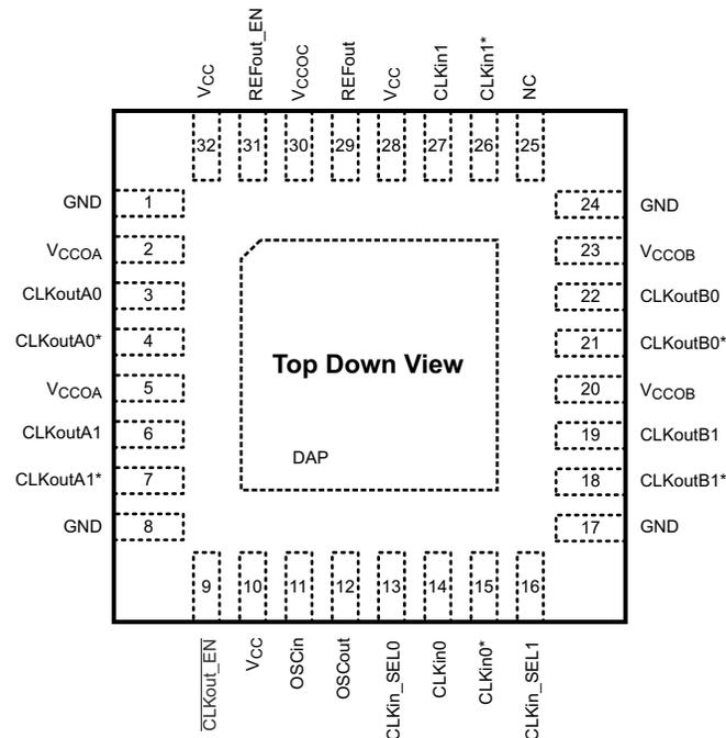
Figure 5-1. RTV Package 32-Pin WQFN Top View
