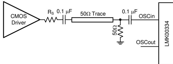
Figure 9-4. Driving OSCin With a Single-Ended Input
