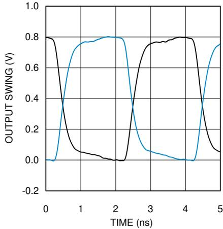
Figure 6-1. HCSL Output Swing at 250 MHz
