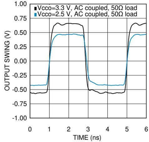
Figure 6-2. LVCMOS Output Swing at 250 MHz
