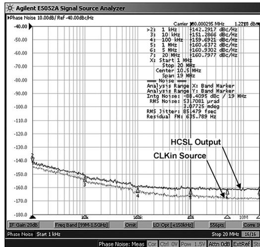
**Figure 6-11. HCSL Phase Noise at 100 MHz**
