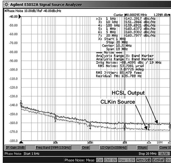
Figure 9-7. HCSL Phase Noise at 100 MHz
