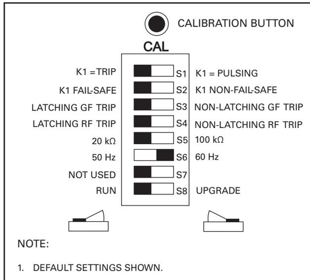
FIG. 1. Configuration switches.
