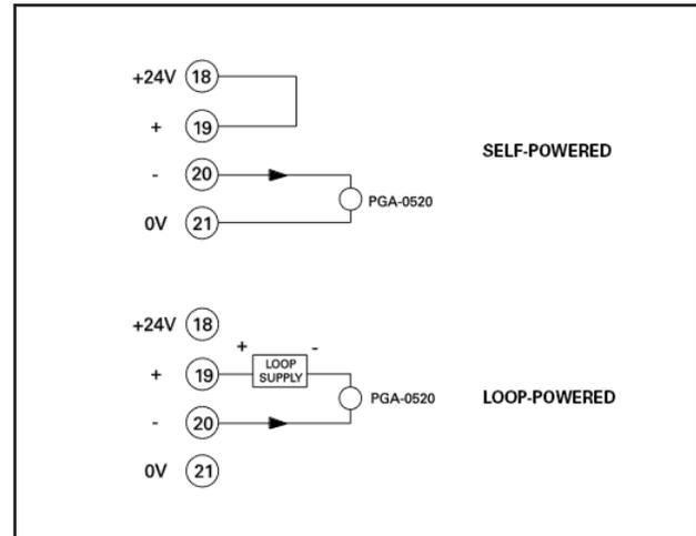
FIG. 2. Analog-output connections.
