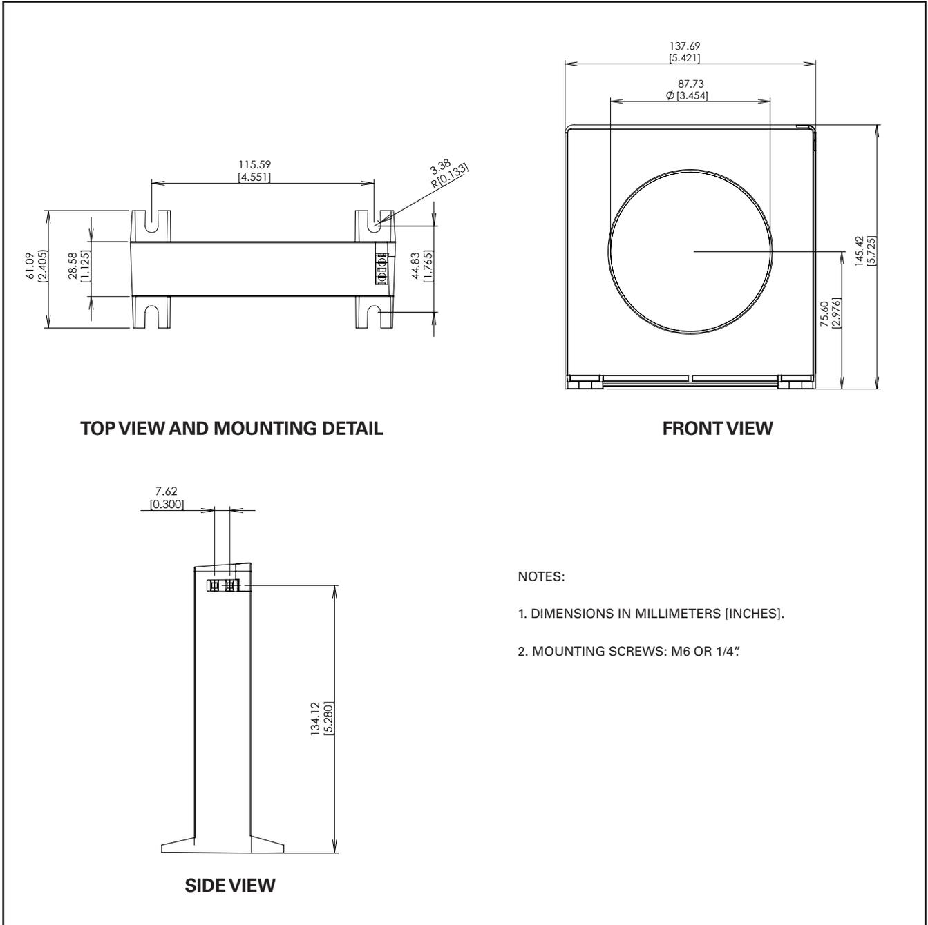
FIG. 16. ELCT5-88 and ELCT30-88 ground-fault current sensors.
