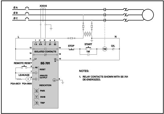
FIGURE 3. Typical Three-Phase-Starter Connection.
