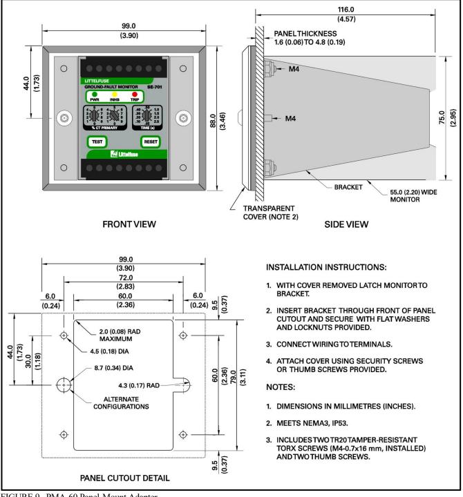
FIGURE 9. PMA-60 Panel-Mount Adapter.
