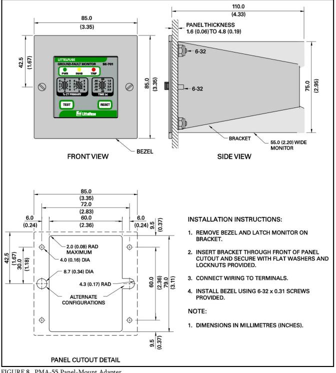
FIGURE 8. PMA-55 Panel-Mount Adapter.
