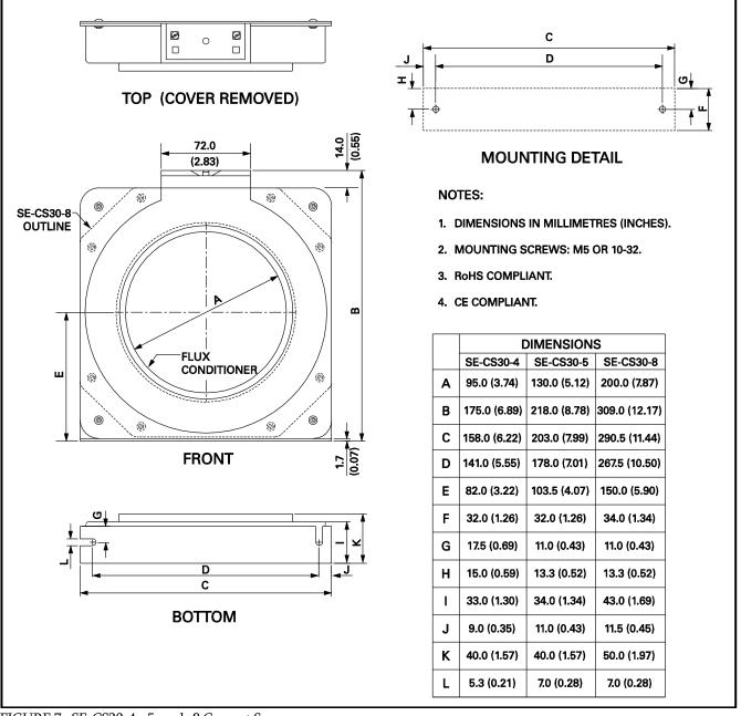
FIGURE 7. SE-CS30-4, -5, and -8 Current Sensors.
