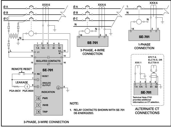
FIGURE 2. Typical Connection Diagrams.
