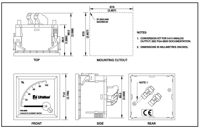
FIGURE 10. PGA-0500 Analog Percent Current Meter.
