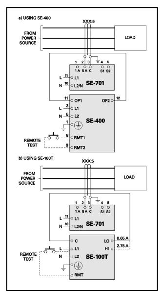
FIGURE 11. Ground-Fault-Test Circuits.
