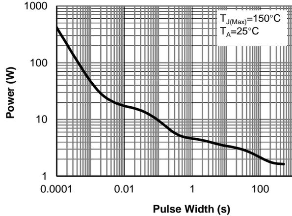
**Figure 10: Single Pulse Power Rating Junction-to-Ambient (Note E)**
