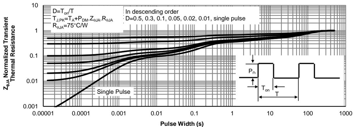
**Figure 11: Normalized Maximum Transient Thermal Impedance (Note E)**
