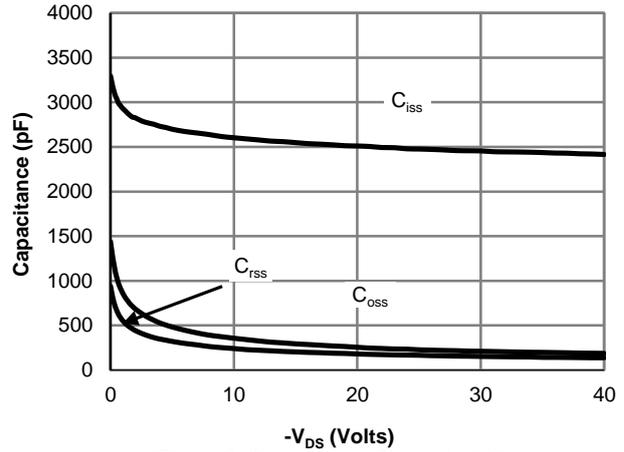
**Figure 8: Capacitance Characteristics**
