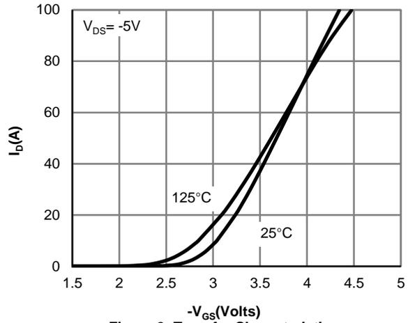
**Figure 2: Transfer Characteristics**
