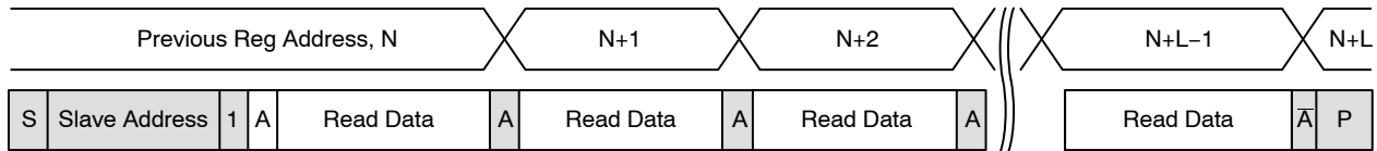
Figure 13. Sequential READ, Start from Current Location
