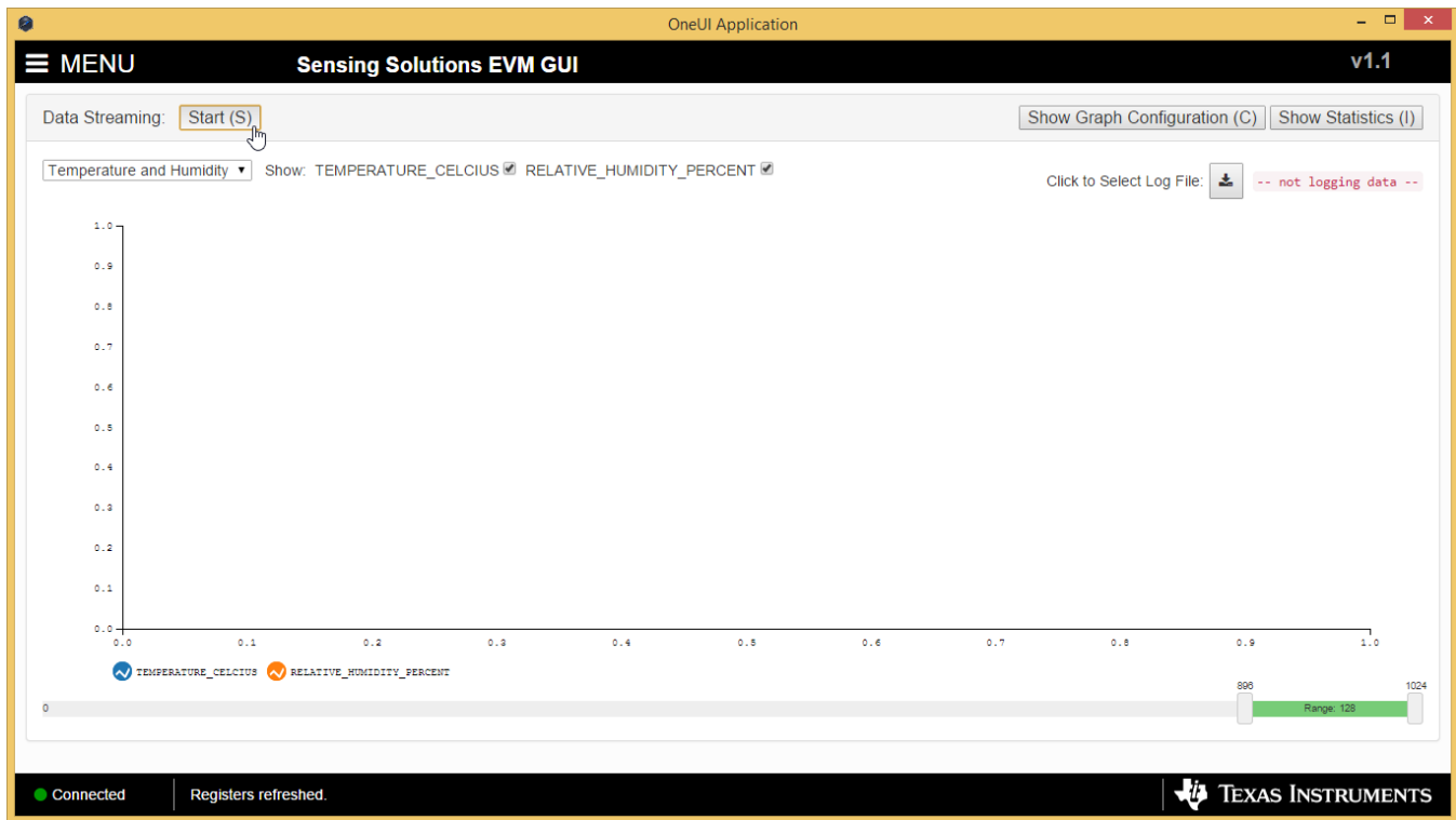
Figure 40. Starting Data Acquisition on Data Streaming Graph
