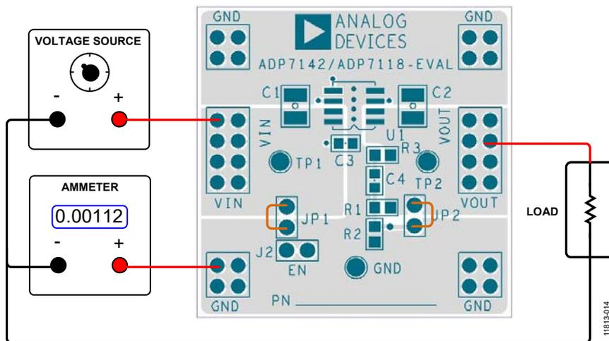
Figure 14. Ground Current Measurement, SOIC
