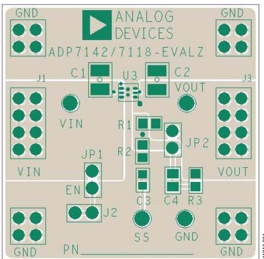
Figure 1. **ADP7118/ADP7142** LFCSP Evaluation Board
