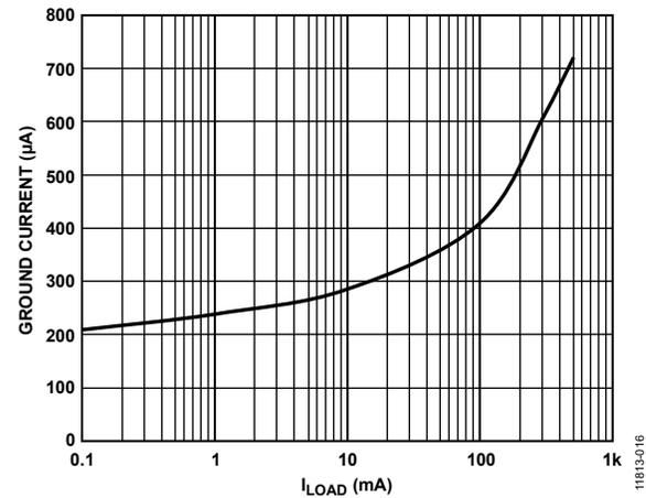
Figure 16. Ground Current vs. Load Current ( $I_{LOAD}$ )
