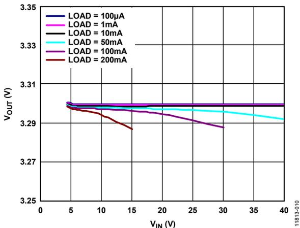
Figure 10. Output Voltage ( $V_{OUT}$ ) vs. Input Voltage ( $V_{IN}$ )
