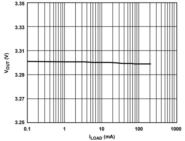
Figure 11. Output Voltage ( $V_{OUT}$ ) vs. Load Current ( $I_{LOAD}$ )
