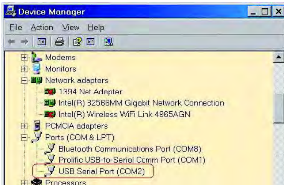
Figure 2. A Successful USB-to-UART Driver Installation
