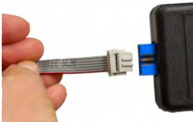
Figure 3. Connecting the Six-Conductor Ribbon Cable to the Serial or USB Smart Cable
