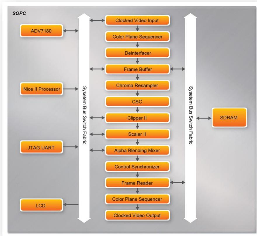
**Figure 4-9 VIP Example SOPC Block Diagram (Key Components)**
