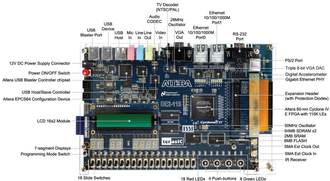
Figure 2-2 VEEK-MT PCB and Component Diagram (bottom view)
