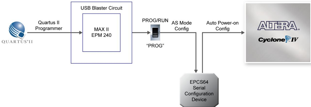
**Figure 3-5 The AS Configuration Scheme**
