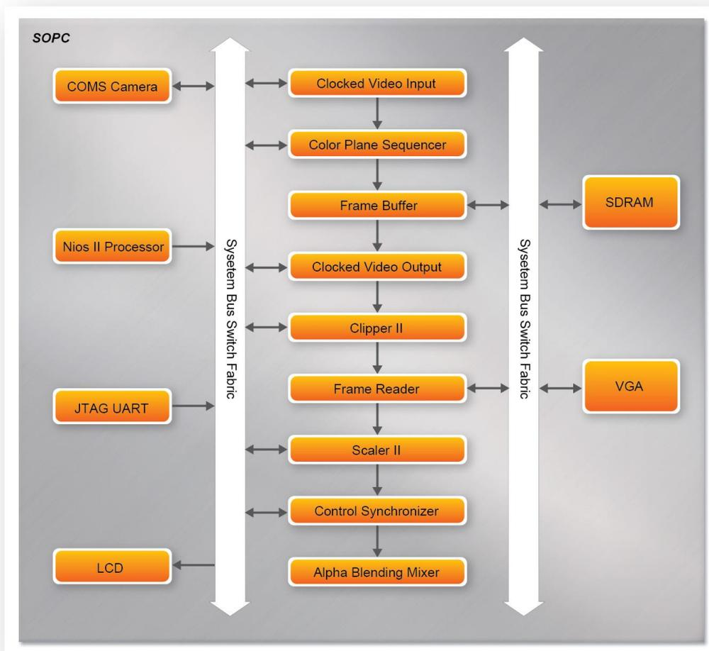
**Figure 4-14 VIP Camera Example SOPC Block Diagram (Key Components)**
